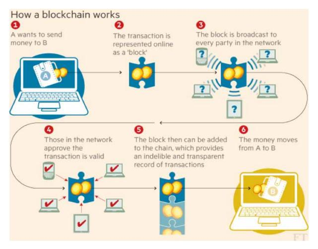
Figure 1.4: Demonstration of a basic blockchain transaction.<sup>27</sup>
